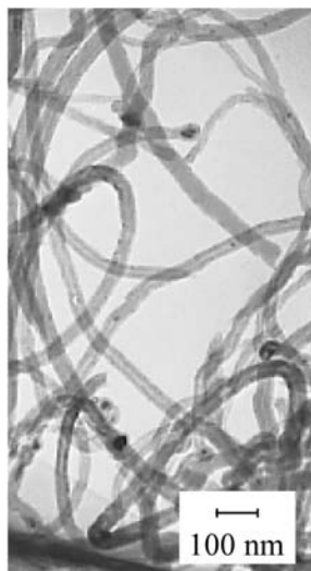
FIGURE 2 TEM image of carbon nanotubes formed on 10 wt% Ni/ZrO 2 (GT).
